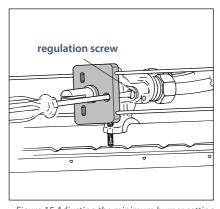
Figure 15 Adjusting the minimum burner setting
